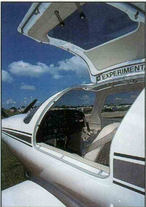
One of the biggest engineering challenges in any pressurized airplane is proper sealing of the cabin door. Note the number of sturdy hooks that are necessary to withstand some 5,000 pounds of pressure on the inside of the Lancair IV-P door.
