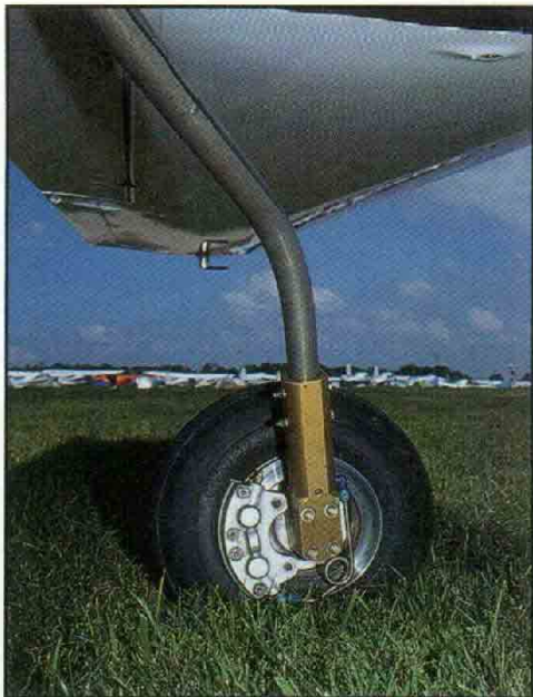
Landing gear detail. Brent used stainless brake lines with loops for added flexibility rather than the standard flexible lines.
