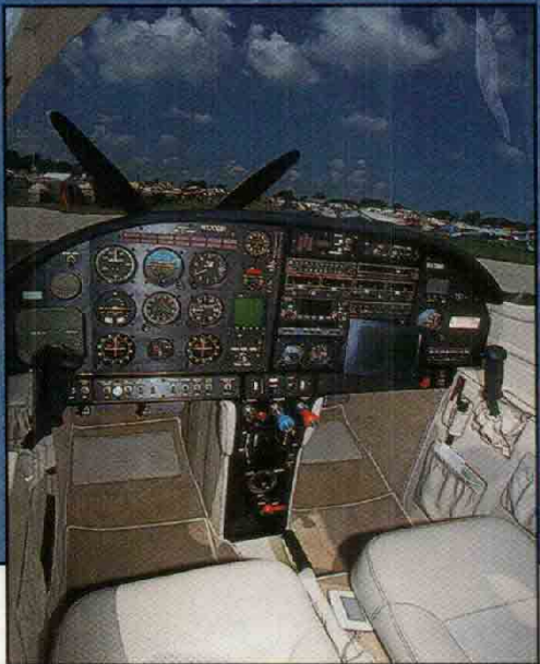
Brent's moving map flight computer is at the lower right of the instrument panel — tilted up 15° for ease of viewing.
