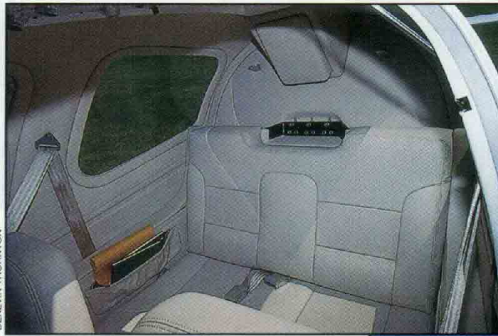
Rear seat of the auto-like cabin. Note the recessed jackbox at the top of the seat back for passenger headsets.
