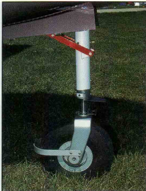
Landing gear detail. Brent used stainless brake lines with loops for added flexibility rather than the standard flexible lines.
