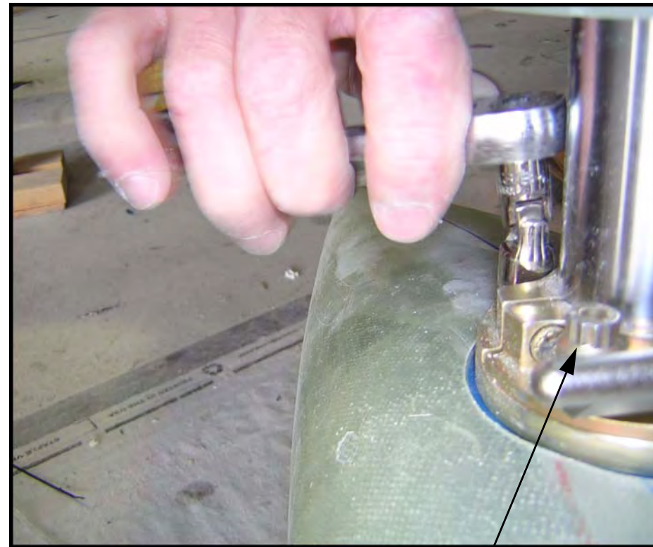
Bolts, MS21250-05015 and MS21250-05013 with countersunk washers, MS20002C5.
