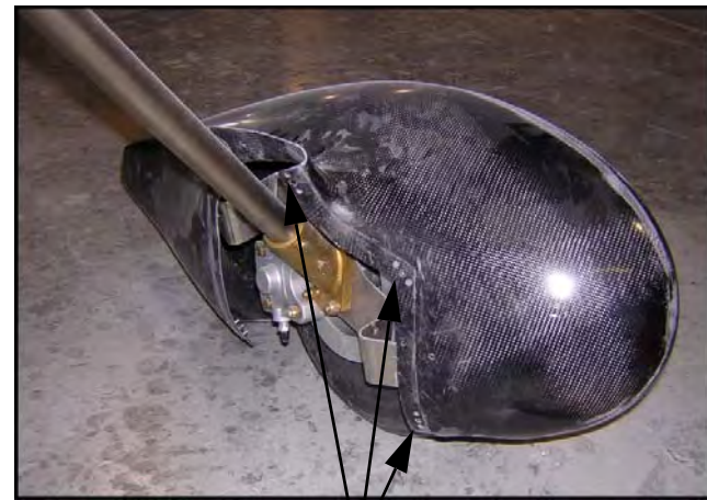
Figure S.5.A.5 Nutplate locations for wheel pant cover
