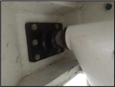
Main landing gear trunnion attach fitting
