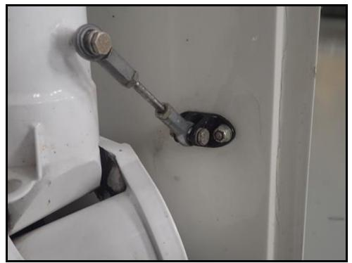
Main landing gear door pushrod attached to landing gear and door
