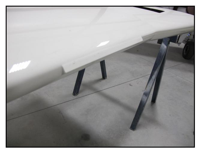
The calibration of the stall warning systems is important for proper function on the aircraft. The Evolution, if it is equipped with stall strips is most likely 14 CFR 23.49 and 14 CFR 23.201, 203 and 207 compliant for stall and stall recovery—if not, it can be a real bad ride. The Lancair IV series aircraft does not appear to have a significant risk of stall accidents once the other factors are understood.
