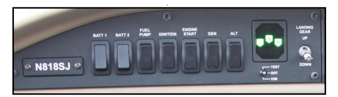
The battery, generator, and the start switches are located on the left brow panel The circuit breakers are located in the circuit breaker box between the pilot and copilot seat or under the power quadrant.
