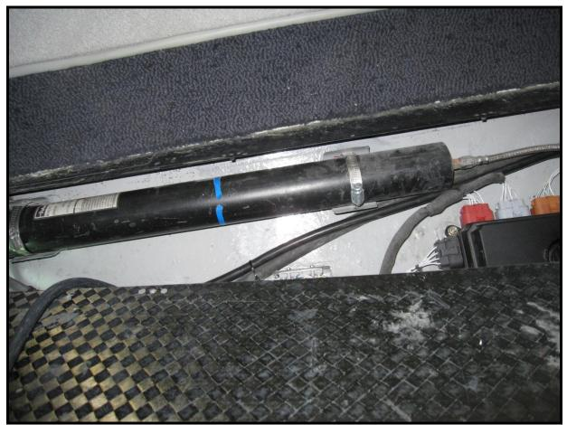
Accumulator A secondary manifold under the pilot seat allows for emergency gear operation.
