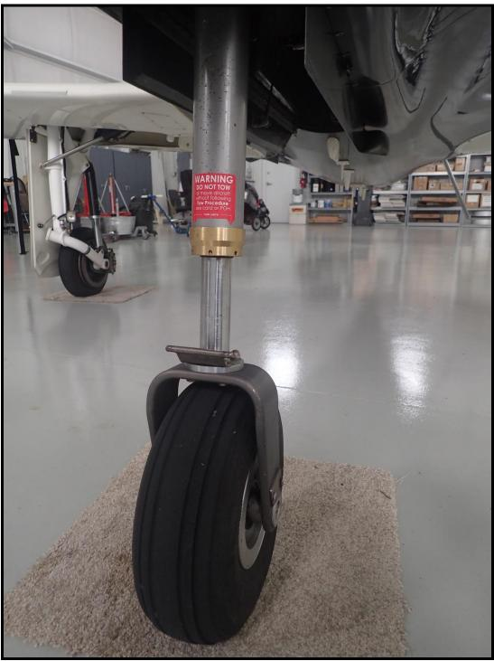
Nose gear strut and wheel and tire assembly
