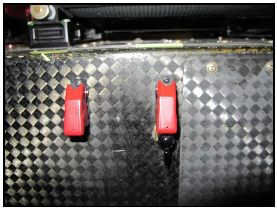
Emergency Landing Gear Hydraulic Valve
