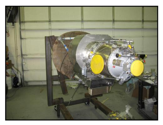
The Pratt & Whitney Canada PT 6A-135A turboprop engine is a reverse flow annular design turboprop engine. The intake air enters at the rear of the engine via the lower cowl intake and engine mounted stainless steel plenum. The plenum is equipped with an electrically operated ice door that when opened by the pilot diverts ice chunks and ingested foreign objects out of the
