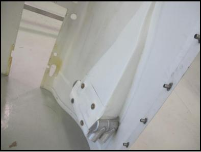
NACA duct with intercooler on right side lower engine cowling
