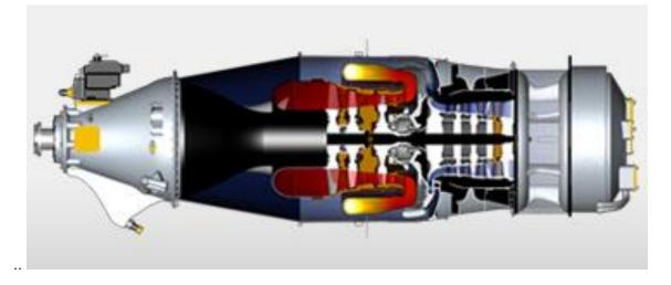
At full power of 1900 rpm; 101,6% NG, 2080 foot pounds of torque the PW&C PT6A-135A develops 750 shaft horsepower. The engine may be operated at maximum power in the climb to cruise altitude. Maximum recommended cruise power setting is 1900 rpm and 805\*C ITT generating 700 shp. A dual igniter provides ignition source for engine starting. An electric fuel pump is installed.
