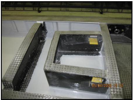
Baffle Tank (shown upside down with gold flapper valves)
