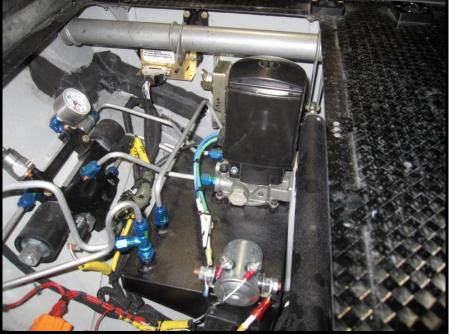
Hydraulic pump, motor and reservoir
