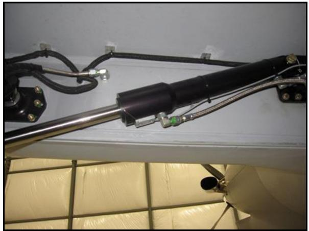
Main landing gear hydraulic actuator
