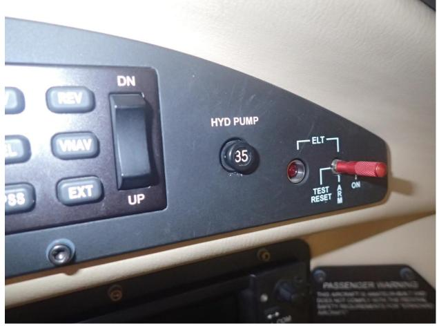
The system is powered through a 35A circuit breaker located on the panel.
