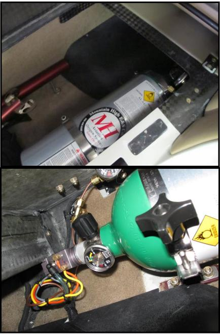
Oxygen Bottle and Regualtor Installed in Aft Bay
