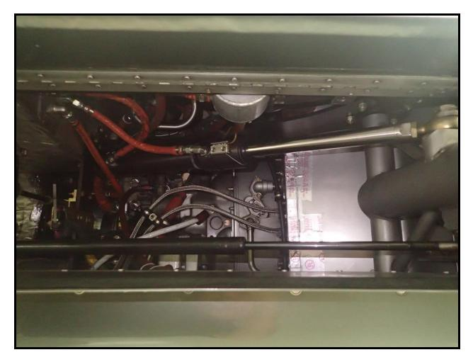
Nose gear actuator (top) and gas strut (bottom)
