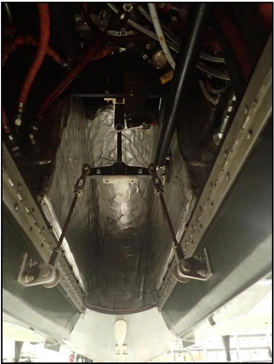
Nose gear tunnel with doors extended
