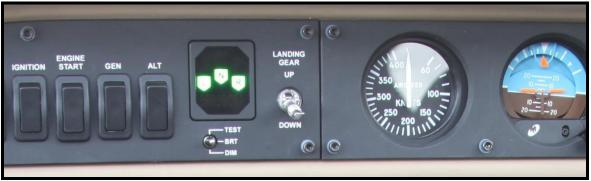
Landing Gear Switch and Indicator
