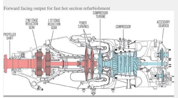
Small and Medium PT6A models incorporate 1-stage axial turbine
