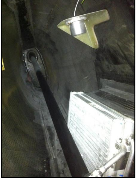
The ailerons and elevator are push rod actuated.
