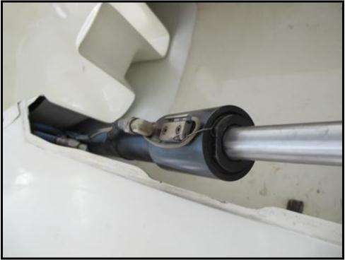
Main landing gear hydraulic actuator with Bimba switch
