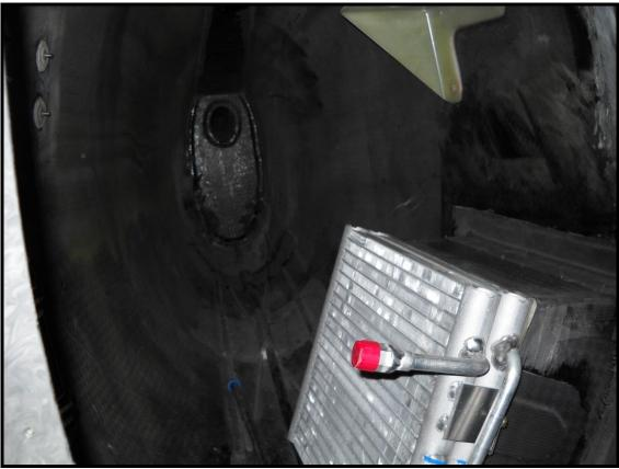
Condenser (mounted behind aft pressure bulkhead)
