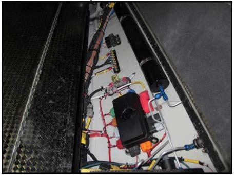
Equipment Bay with Hydraulic Pump, Reservoir, and Accumulator
