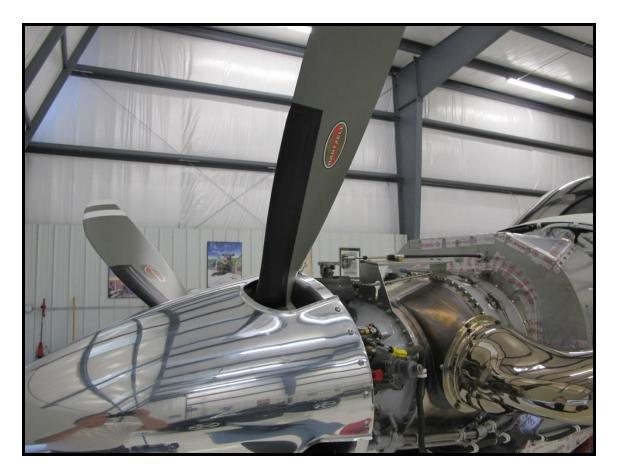
A deice ring and block assembly provide electrical power to the heated boots on the propeller. The carbon blocks require inspection every 100 hours of operation and replacement as necessary.
