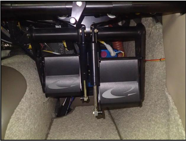
Co-pilot adjustable rudder pedals
