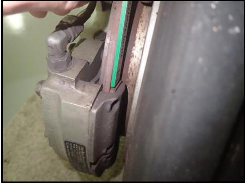
Checking brake pads for wear thickness with a Cleveland "no go" guage (green)
