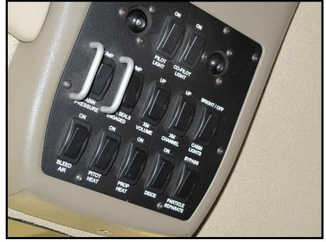
Engine "bleed air" is taken from the compressor stage of the engine and routed through an intercooler on the right side of the lower engine cowl before it goes to the "flow pack" on the forward side of the fire wall. The purpose of the flow pack is to reduce pressure and temperature.
