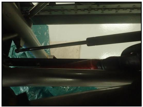
Nose gear gas strut
