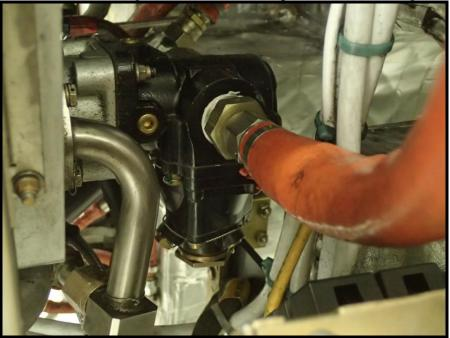
Mechanical Engine Drive Fuel Pump on Engine Accessory Pad
