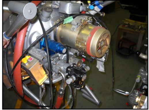
A 300 ampere gear driven starter generator is mounted on the rear accessory case of the engine.
