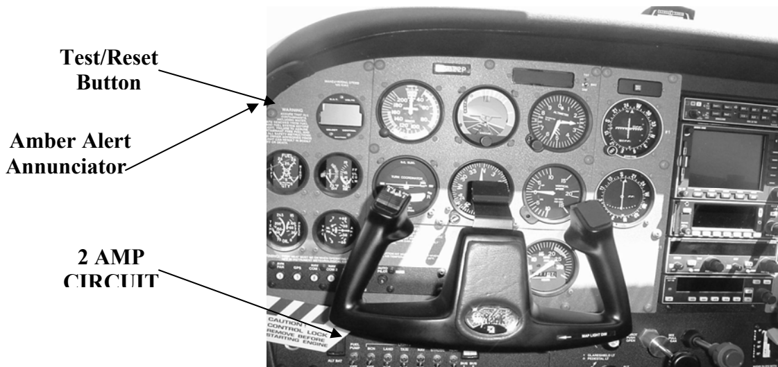
FIGURE 2 - TYPICAL PILOT INSTALLATION SHOWN
